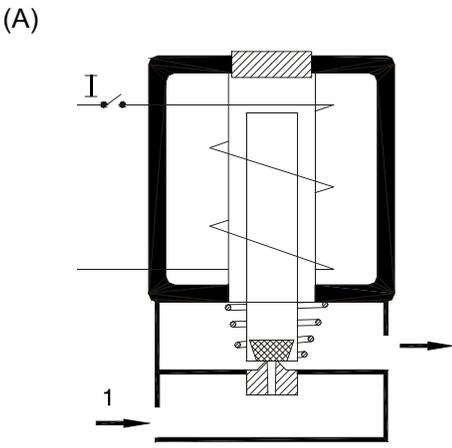
The Solenoid is directly responsible for opening and closing the ports and thereby controlling the direction of fluid flow in the Direct Acting Solenoid Valve.
