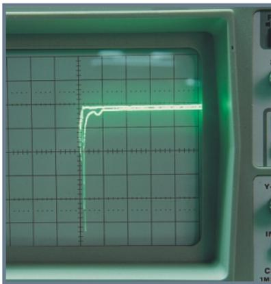
Any solenoid is an energy storing device and each time it is deenergised the energy is released in circuit in the form of a surge which may affect the switching circuit. Higher the power consumption of the solenoid, higher is the surge. **ROTEX** uses solenoids with a maximum of 11 Watt power consumption. In order to absorb the surge, **ROTEX** uses a surge suppressor device in all solenoids above 10 Watt power consumption and in all Flameproof / Explosionproof solenoids as a standard.
