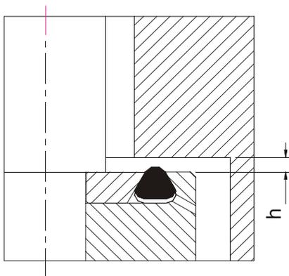
A small movement of the poppet ( $h$ ) creates a large opening equal to the orifice. As a result, the poppet operates within a time of 10 ms to 40 ms (depending on the size of the Pilot Operated Solenoid Valve). Each time the valve is operated, a self cleaning action takes place.
