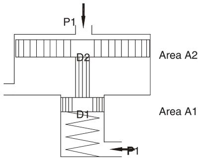
The Poppet Technology works on the differential area principle. As illustrated in the figure here, on energisation, pressure  $P_1$  is acting simultaneously on both areas  $A_2$  ( $\propto D_2^2$ ) and  $A_1$  ( $\propto D_1^2$ ). However, as a result of the area  $A_2$  being larger than  $A_1$ , the entire assembly experiences a downward force which moves the assembly downward. On deenergisation poppet moves up due to spring and pressure on area  $A_1$ .
