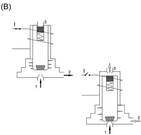
On energising the Solenoid, the electromagnetic field generated pulls the plunger thereby blocking orifice at Port-3 and opening passage from Port-1 to Port-2.
