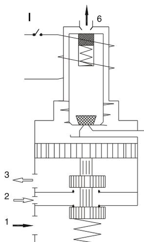
When pressure is applied at inlet port, a part of media from the inlet is drawn under the plunger through the pilot passage.
