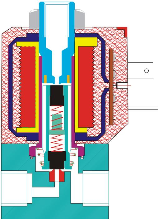
All **ROTEX** solenoids are constructed with magnetic path enclosures surrounding the basic solenoid. As a result, in a **ROTEX** solenoid, all the generated electro magnetic flux is used in order to lift and hold the plunger. **ROTEX** solenoid valves offer higher pressure to orifice rating with a lower power consumption. Thus, demonstrating the highly efficient solenoid design and operation.
